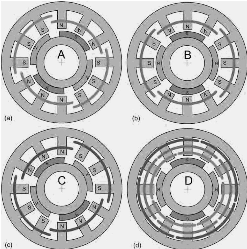
**Figure 1-11.** A motor with distributed windings.
