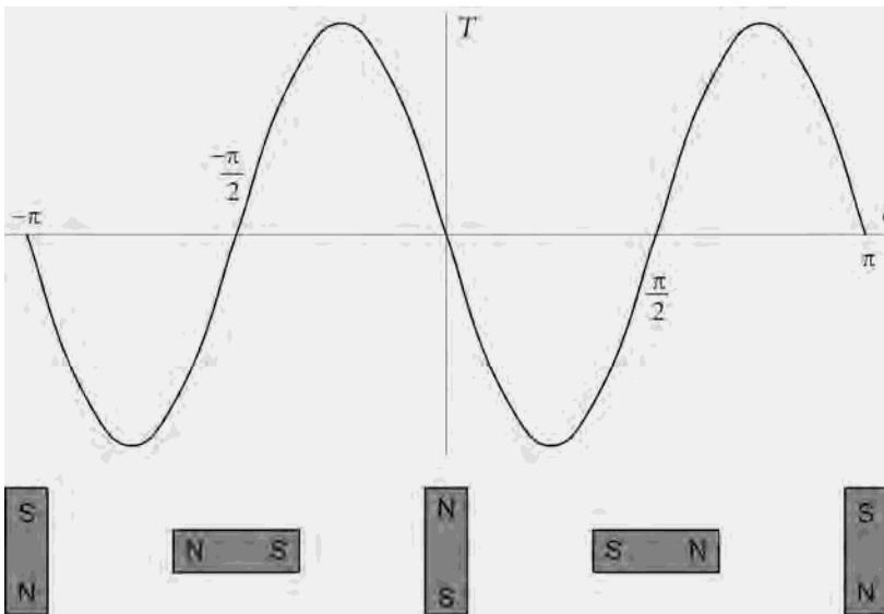
**Figure 1-7.** Torque experienced by the magnet in Fig. 1-6.
