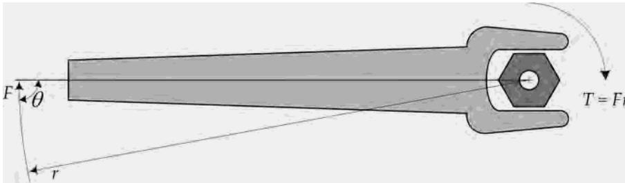
Figure 1-4. A wrench on a nut.
