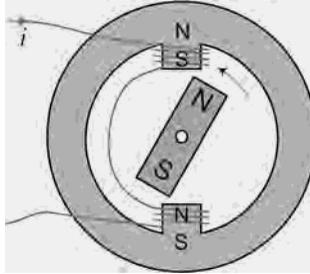
**Figure 1-8.** Current-carrying windings added to Fig. 1-6.
