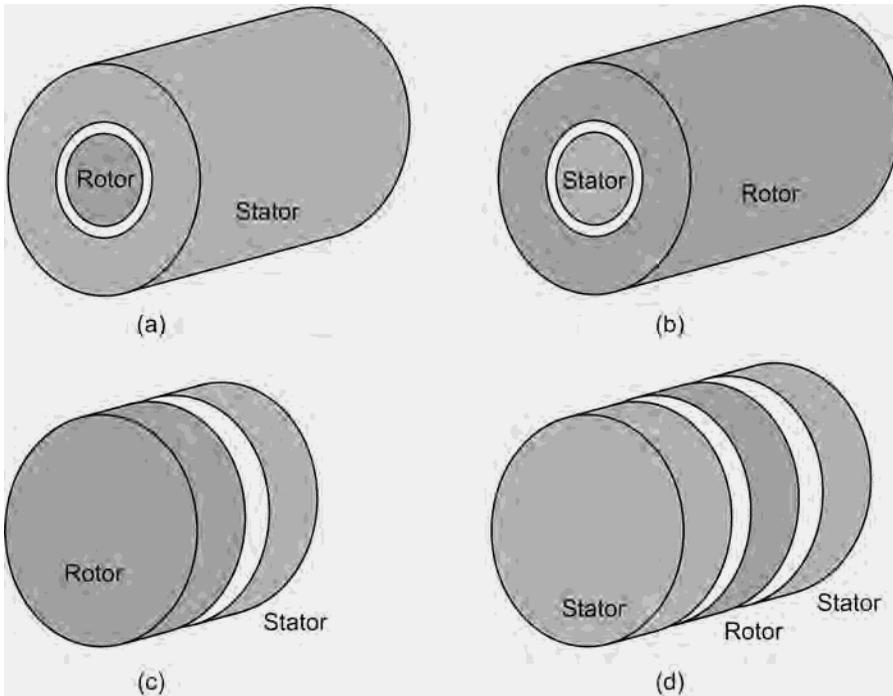
**Figure 1-2.** Some motor construction possibilities.
