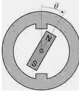
**Figure 1-6.** A magnet free to spin inside a steel ring having two poles.
