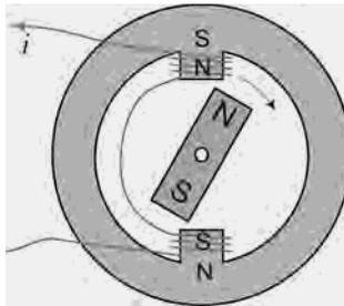
**Figure 1-9.** Current flow in the opposite direction compared to Fig. 1-8.
