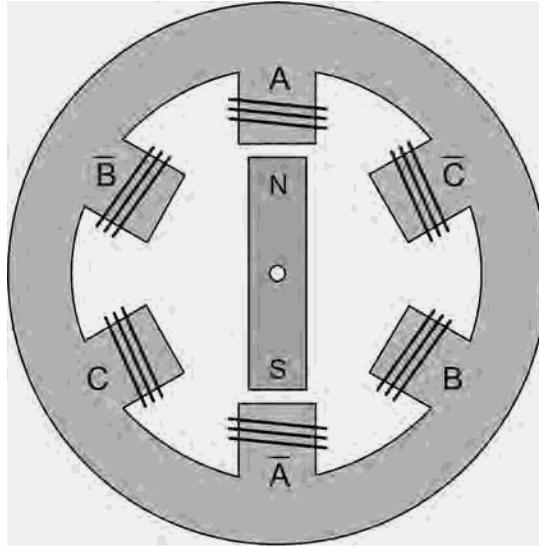
**Figure 1-10.** A motor having three phases.
