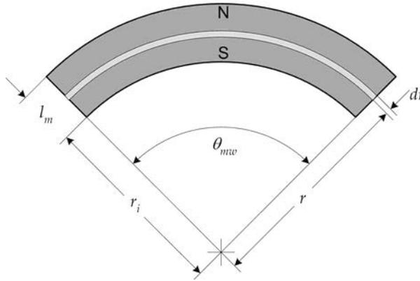
**Figure 2-22.** An arc-shaped permanent magnet magnetized radially.
