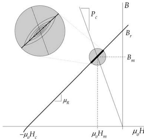
**Figure 2-20.** Dynamic operation of a permanent magnet around an operating point.
