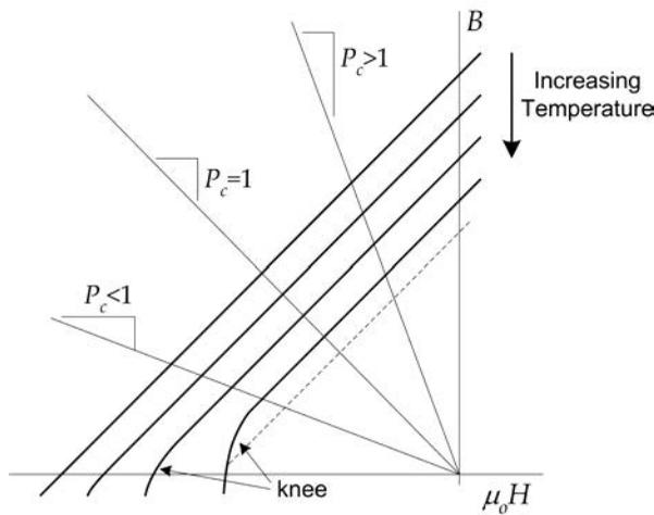
**Figure 2-19.** Influence of temperature on the demagnetization curve.
