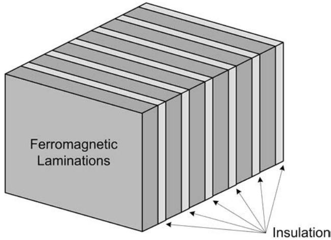
**Figure 2-16.** Laminated ferromagnetic material.
