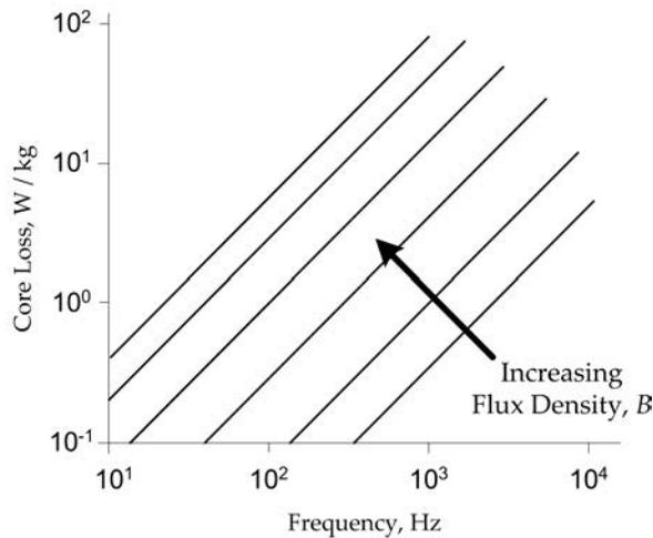
**Figure 2-15.** Typical core loss characteristics.
