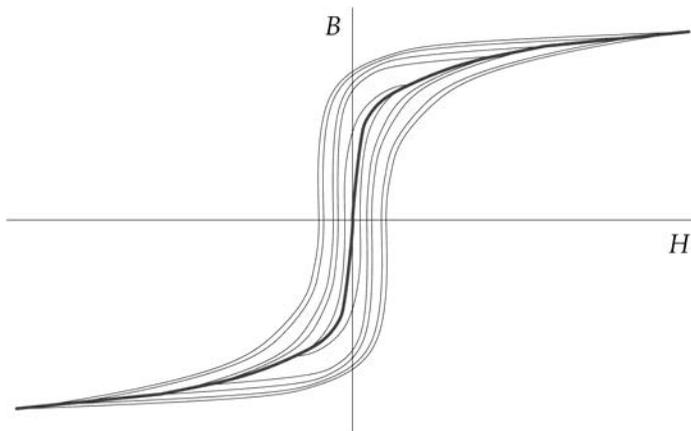
**Figure 2-14.** Typical ferromagnetic material magnetization characteristics.
