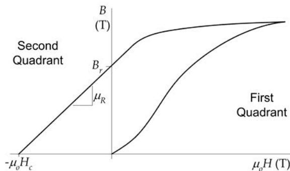
**Figure 2-17.** The  $B$ - $H$  loop of a permanent magnet.
