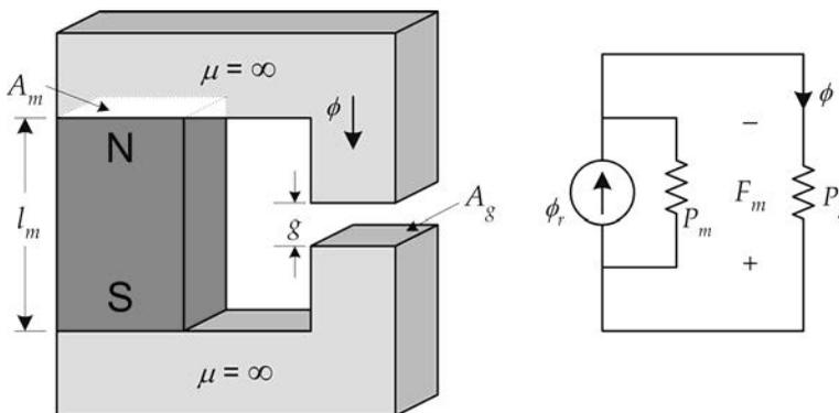
**Figure 2-23.** A simple magnetic structure and its magnetic circuit model.
