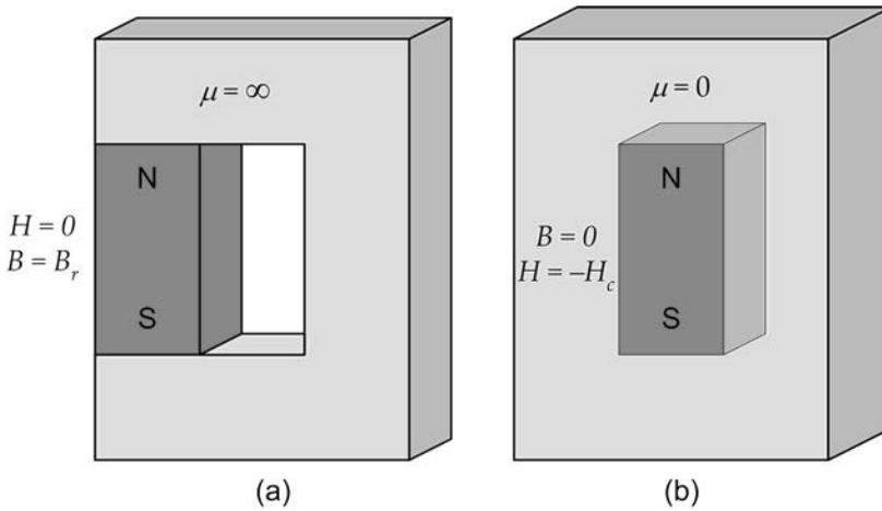
**Figure 2-18.** Operation of a permanent magnet at its (a) remanence, and (b) coercivity.
