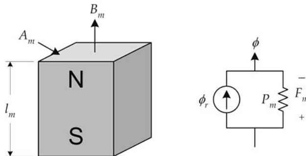
**Figure 2-21.** A rectangular permanent magnet and its magnetic circuit model.
