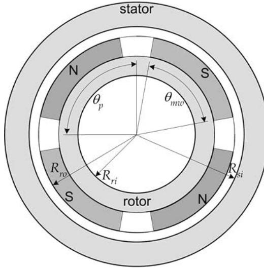
**Figure 6-1.** A rotor having surface mounted magnets.
