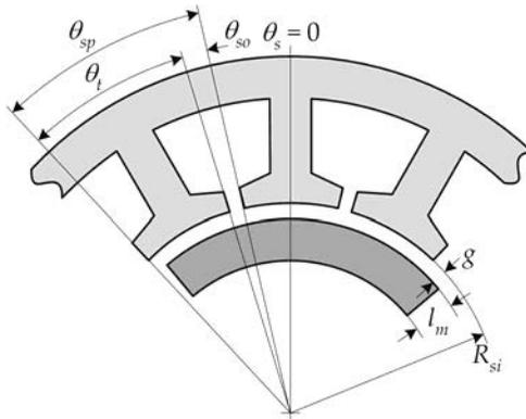
**Figure 7-2.** Geometry for the computation of the slot correction factor.
