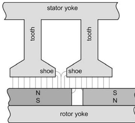
**Figure 7-1.** Representative permanent magnet flux flow pattern.
