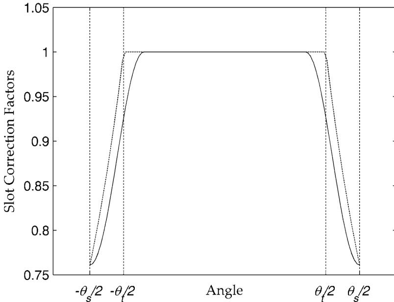
**Figure 7-3.** Slot correction factor illustration.
