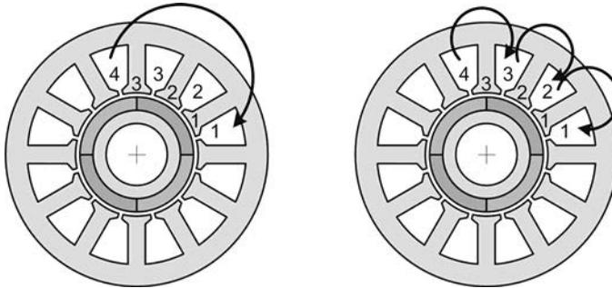
**Figure 7-4.** A coil and its single tooth equivalent.
