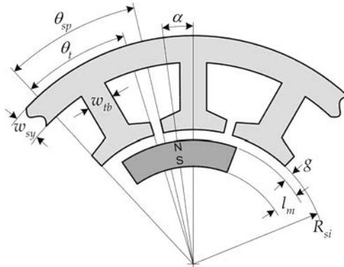
**Figure 7-5.** Geometry for the computation of tooth flux.
