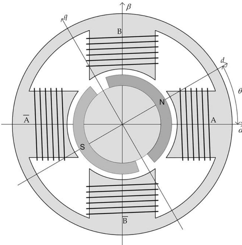
**Figure 10.1** A conceptual two phase motor.
