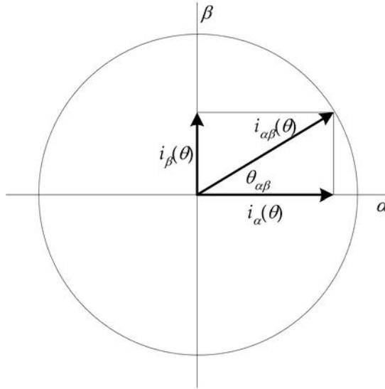
**Figure 10-3.** Graphical definition of space vectors in rectangular and polar forms.
