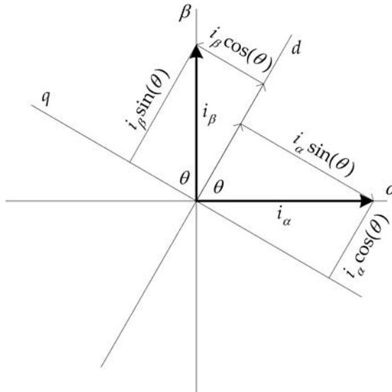
**Figure 10-4.** Park transformation relationship between the stator and rotor coordinate systems.
