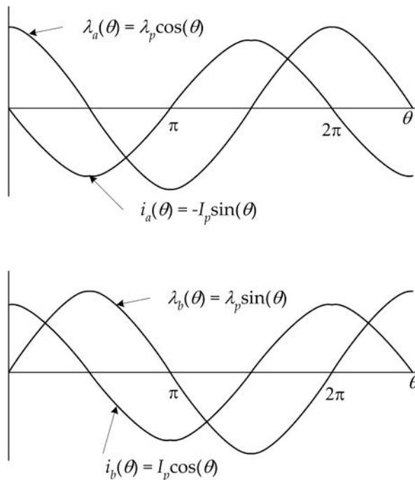
**Figure 10-5.** Relationship between currents and flux linkages.
