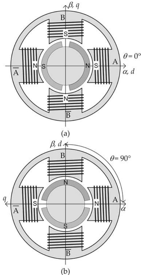
**Figure 10-2.** A conceptual two phase motor with the rotor position at (a)  $0^\circ$ , and (b)  $90^\circ$ .
